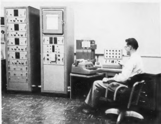
Any desired number of SADIC channels may be combined. The above system contains 4 channels and readout devices.
